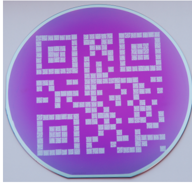
FIGURE 5.5 – Design of the HDP disk. Each pixel in the large QR codes consists of a QR code.
